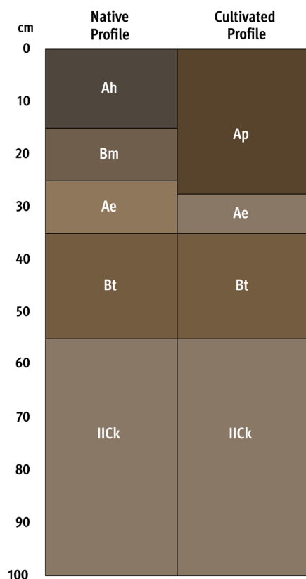
Figure 8. A typical Guelph soil series profile under native and cultivated land use. Note the surface horizons from the native land use are homogenized into an Ap (p = plowed) horizon under agricultural land use.
